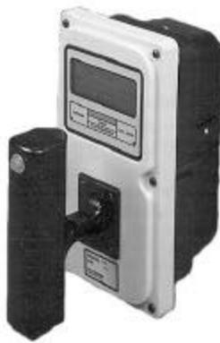
The Model 450 Ion Chamber Survey Meter is a lightweight hand-held, battery operated unit designed to measure alpha above 4 MeV, beta above keV, and gamma and x-ray radiation above 7 keV, using the latest CMOS and LCD technology.
